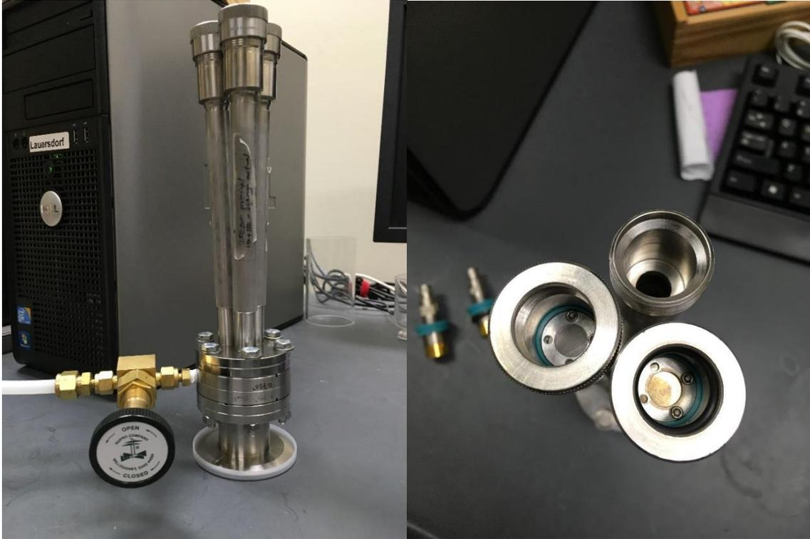
Figure 2.1 (a) The exterior housing with both the CF 2  $\frac{3}{4}$  to KF 50 and vacuum pump-out attached.
