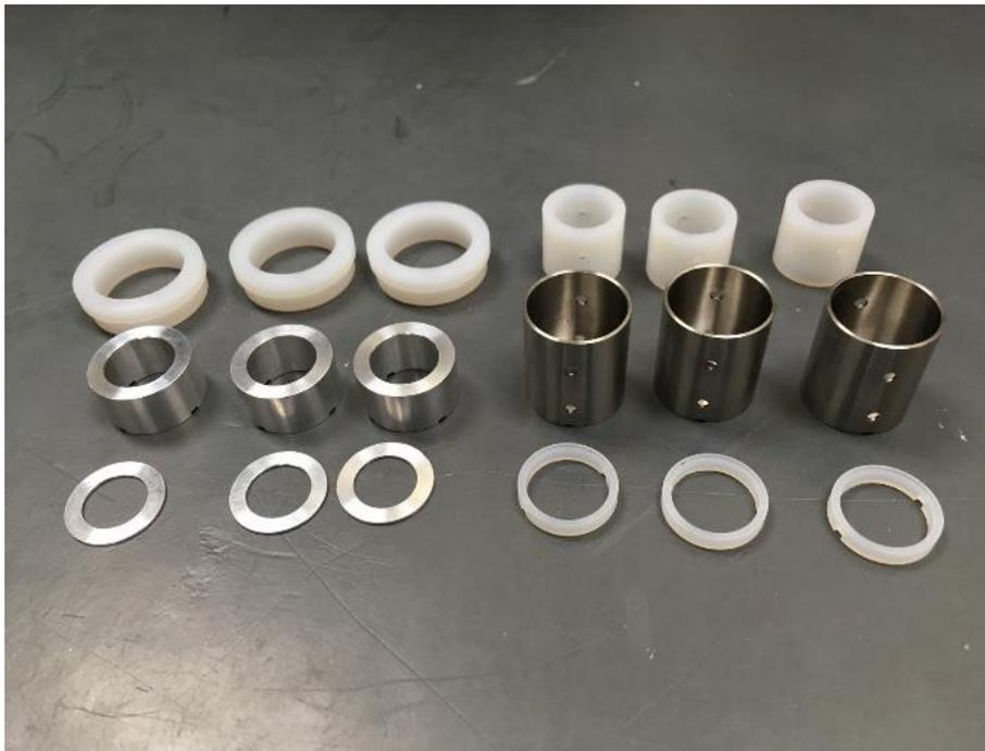
Figure 2.6: In-house manufactured inner housing components. The opaque white pieces are made from turcite for grounding purposes. The thin aluminum disk is the filter mount. These do not have filters on them and were designed for test fitting purposes due to the fragility of the filters.
